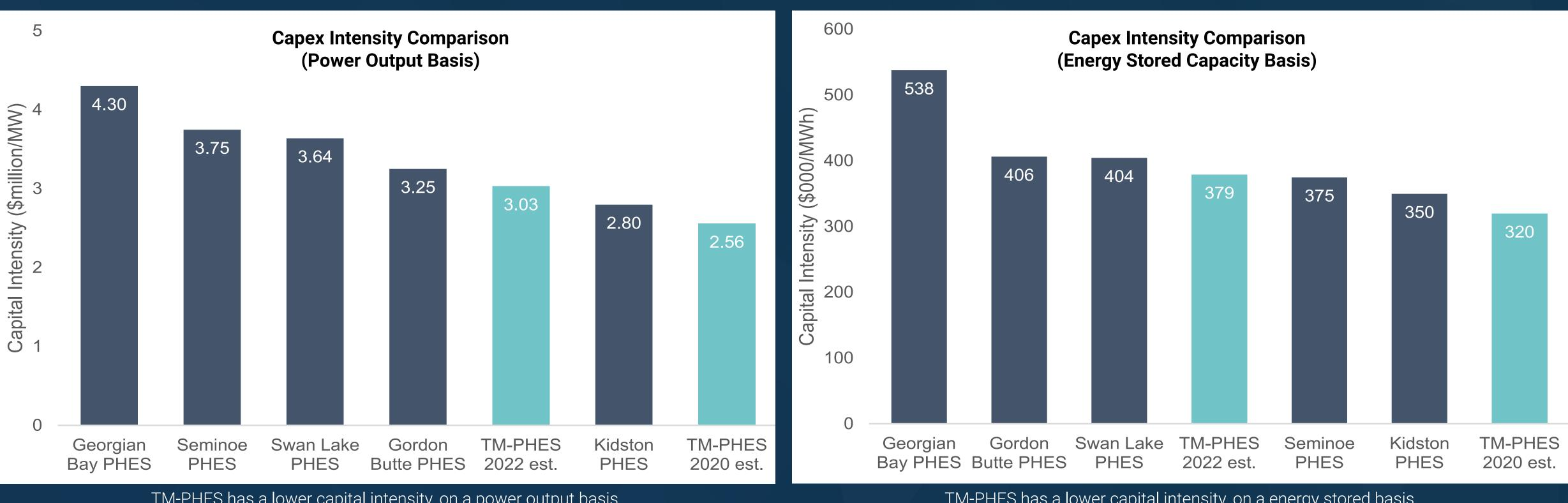
TM-PHES has a lower capital intensity, on a power output basis, than similar PHES projects in North America.
